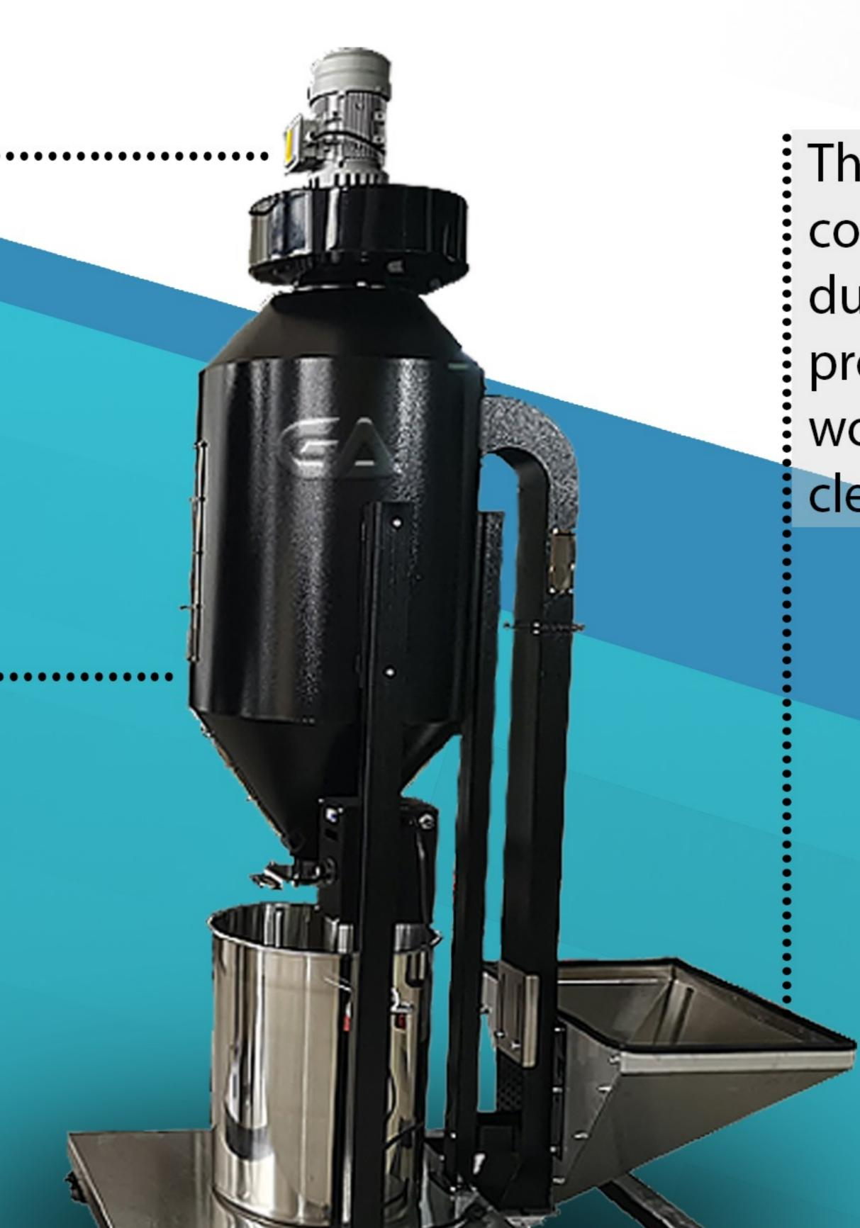
The Side Cyclone Dust collector captures dust during the destoning process and keeps the working environment clean.
